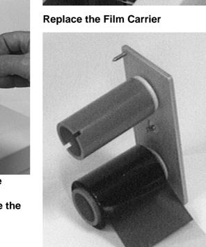
Open the Dye Film package. Fit the dye film on the lower boss, observing the
